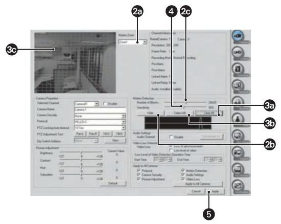
Figure 93. Camera Motion Detection Setup
